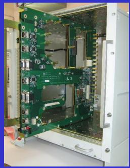
•To support switching of hundreds of high speed radio channels at baseband (Up to 2 GBps links).
