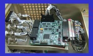
•Rear unit supports COM Express processing unit (Intel ATOM Z530 Vxworks OS) application boards, RS422 communication ports, and power.
