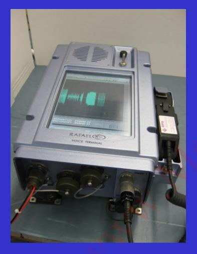
•Touch screen LCD display. •Conduction cooling. •State of the art COM-Express processing module (Intel ATOM Z530). •Custom carrier developed by us supporting audio, handsets, backlight control, touch control & power.
